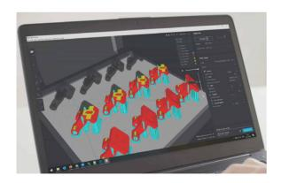
BLADE, BigRep's easy to use slicer software, allows for greater control of printing parameters on all BigRep large-format 3D printers. Its integrated estimation engine gives accurate printing time and material use predictions for unmatched planning and productivity.
