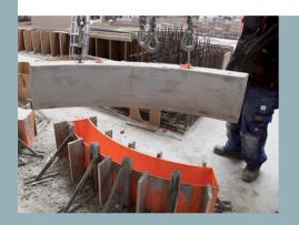
3D printed patterns and molds can replace expensive CNC milled or hand-crafted traditional forms. By modernizing the first phases of numerous casting applications, the BigRep ONE allows you to produce in-house, iterate faster, cut material costs, and streamline logistics. BigRep customers use the ONE to print forms for making carbonfiber parts like drones and custom auto bodies, for various kinds of concrete casting, and to produce patterns for anything from bathtubs to propellers.
