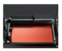
Preparation time is significantly reduced for all print projects by the fast-heating print bed. Capable of quickly reaching 100 °C for optimal print bed adhesion with a variety of high-quality materials. An inductive sensor enables semi-automatic print bed levelling to ensure optimal calibration and maximum control.
